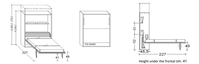
With the electric opening it is NOT possible have the drawers under the bed. Instead of the drawers there will be a fix band.
