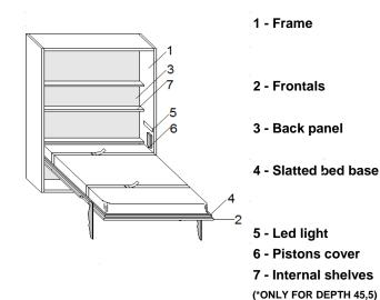
Panel of wood agglomerate in conformity with CARB II, veneered with laminate, wood or lacquered colours.
